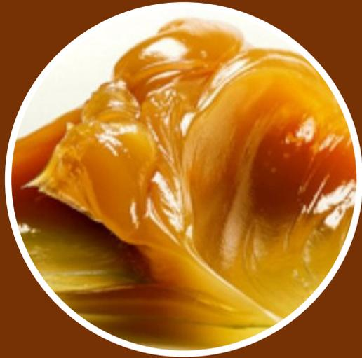
Thickeners - In simple words thickeners are the thickening agents for oil. Thickeners help to turn oil into grease and make it easier to apply on the equipment where oil can't be applied. Thickener is a material that, in combination with the base oil, will produce the solid to semi-fluid mass i.e grease.
